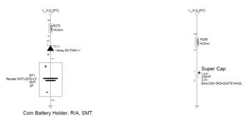
Figure 34 RTC Battery
