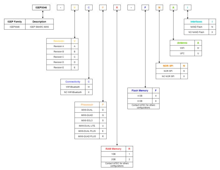
Figure 1 IGEP™ SMARC iMX6 Possible Part Number
