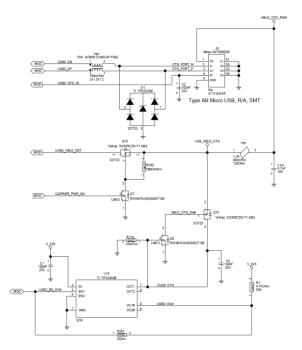
Figure 20 MicroUSB AB 2.0 OTG connections
