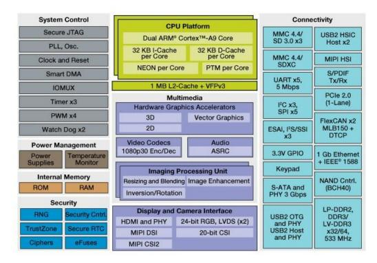
Figure 6 NXP iMX6-DUAL Processors Block Diagram
