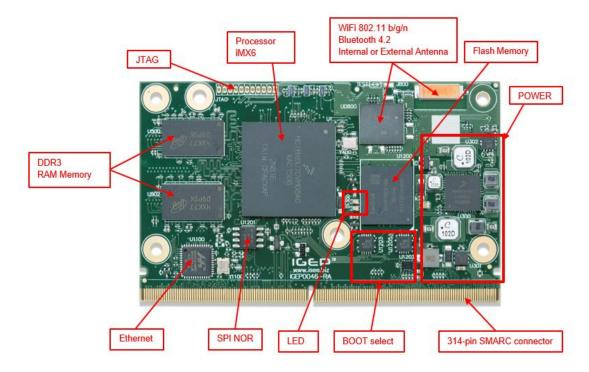
Figure 5 SMARC iMX6 Components Map
