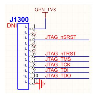
Figure 40 JTAG connector schematic
