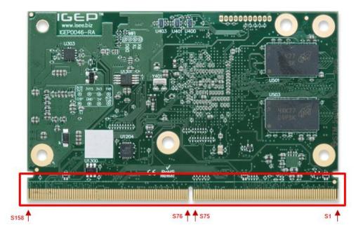
Figure 13 SMARC interface area (BOTTOM Side)
