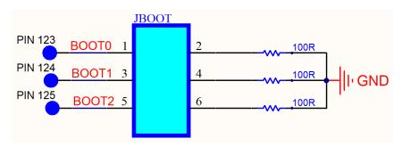
Figure 16 Boot Mode: jumpers selectors
