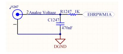
Figure 33 PWM example: RC filter
