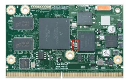
Figure 38 LEDs position in the PCB
