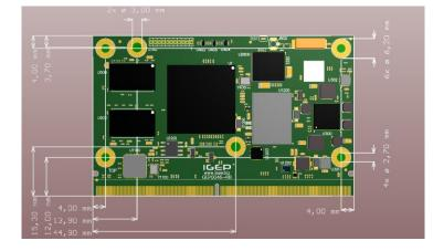
Figure 37 IGEP™ SMARC iMX6 side view detailed mechanical dimensions
