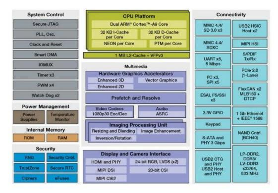
Figure 10 NXP iMX6-DUAL PLUS Processors Block Diagram
