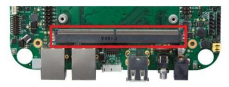
Figure 14 SMARC CONNECTOR
