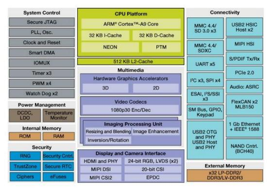
Figure 8 NXP iMX6-SOLO Processors Block Diagram
