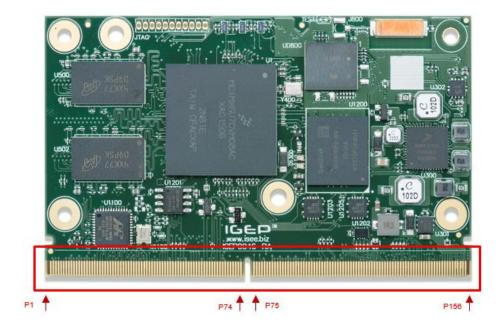
Figure 12 SMARC interface area (TOP Side)
