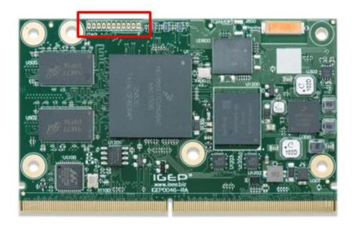
Figure 39 JTAG position in the PCB
