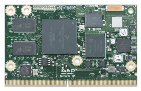
Figure 2 SMARC iMX6 - Top View
